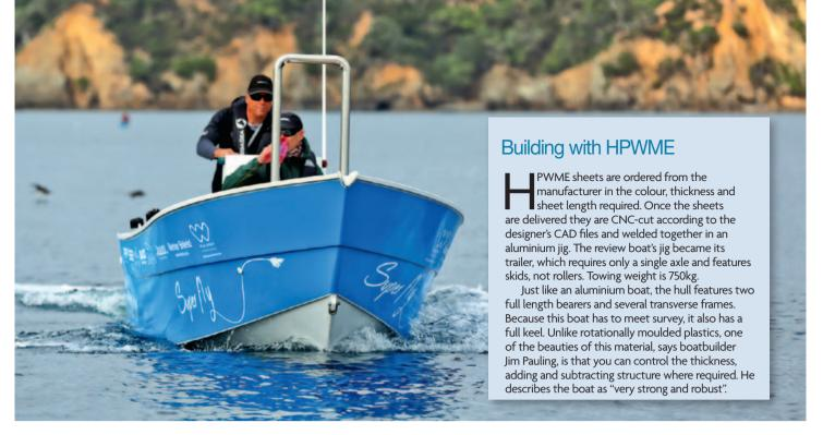
Pauling chose HMWPE construction because it's a robust material able to withstand the general wear and tear that goes with charter fishing. The boat could equally well be constructed using aluminium, timber or composite panels.
