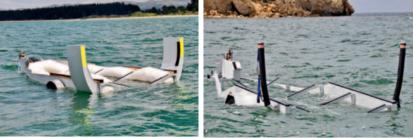
Both trailers floating at anchor, Bill's with additional buoyancy provided by a bladder system he can inflate with an electric pump, plus aluminium 'wings' over the guide poles
