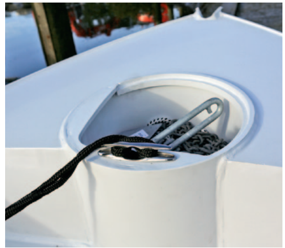
Left: There is plenty of room for larger items under the casting platform, while the suspended storage mesh takes care of smaller items. Right: The anchoring system is very simple; a drogue can also be deployed from the recessed cleat to the rear.
