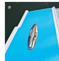
Top left: Railblaza Starport receptacles are spread around the boat and will accept a wide range of accessories. Top right: Cleats are retractable – if a flyline can snag on anything it will!
