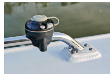
Top left: Railblaza Starport receptacles are spread around the boat and will accept a wide range of accessories. Top right: Cleats are retractable – if a flyline can snag on anything it will!
